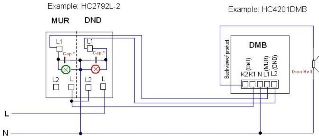
Cap.\* - Add 0.15uF/0.22uF,275VAC X2-Safety Capacitor across LED indicator if there is residue voltage issue
